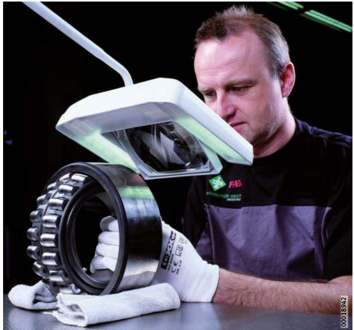
Figure 6 Bearing examination by Schaeffler reconditioning specialists
