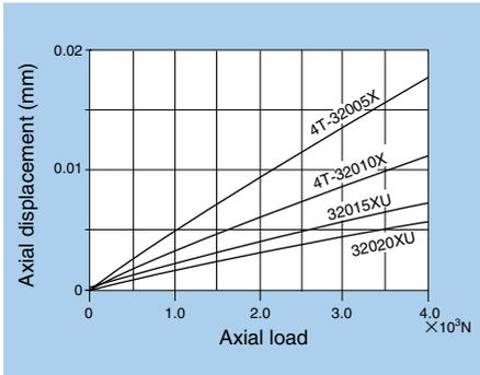
Fig. 9.6.1 Axial Load and Displacement for 320 Series
