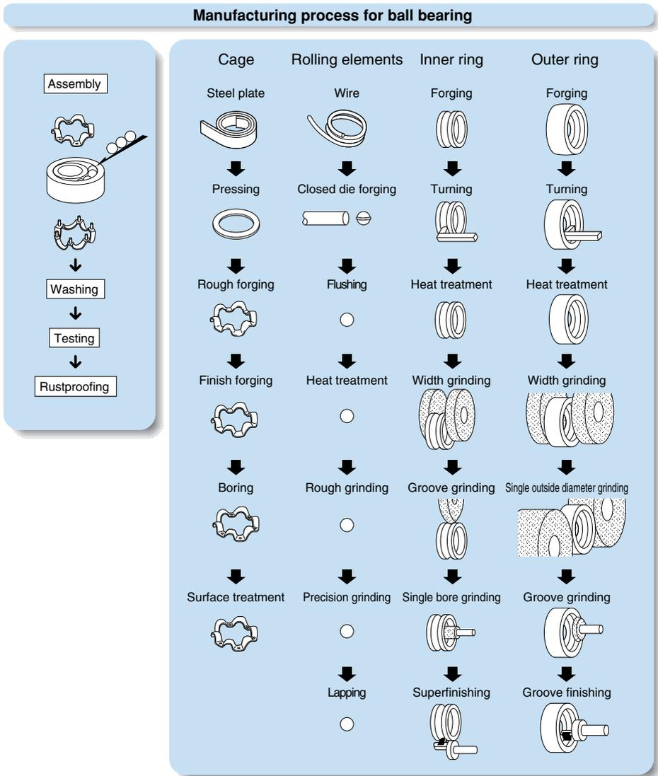
Fig. 2.4 Deep Groove Ball Bearing Manufacturing Process
