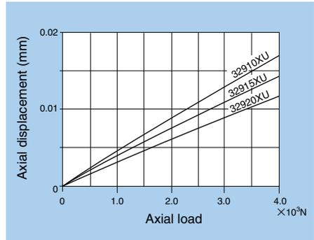
Fig. 9.6.2 Axial Load and Displacement for 329 Series
