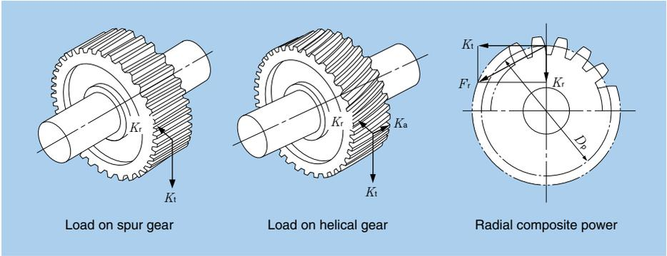
Fig. 7.1 Load on Gears
