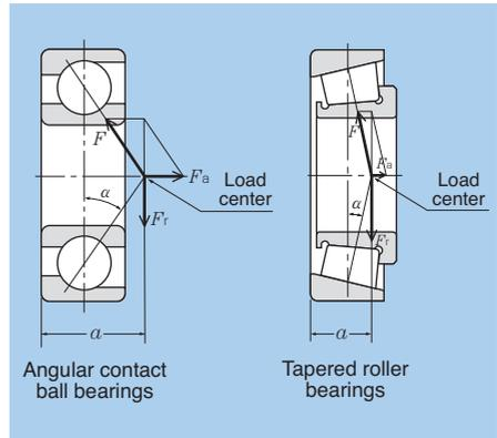
Fig. 7.4 Pressure Cone Apex and Axial Component Force
