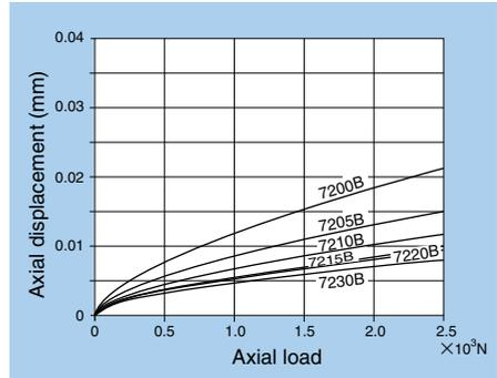
Fig. 9.5.8 Axial Load and Displacement for 72B Series
