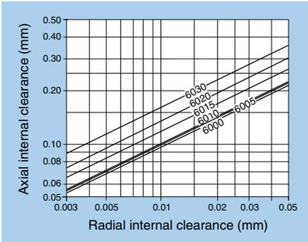
Fig. 9.4.3 Axial and Radial Internal Clearance for 60 Series
