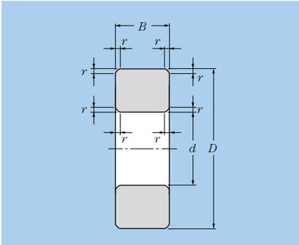
**Fig. 4.1 Radial Bearing** (tapered roller bearings not included)
