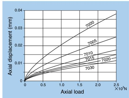
Fig. 9.5.4 Axial Load and Displacement for 70 Series
