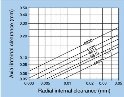
Fig. 9.4.1 Axial and Radial Internal Clearance for 68 Series
