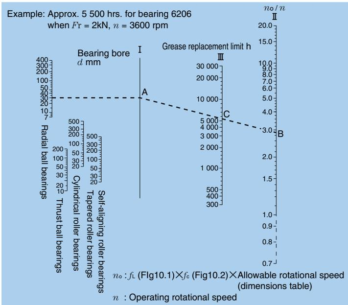
**Fig. 12.3 Diagram for Determining Grease Replenishment Interval**
