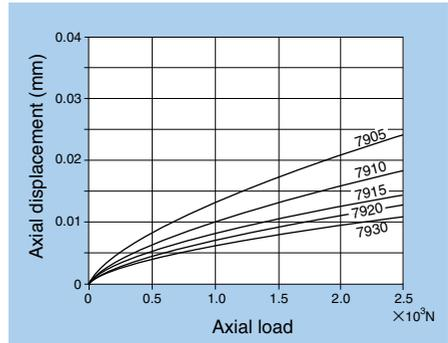
Fig. 9.5.2 Axial Load and Displacement for 79 Series
