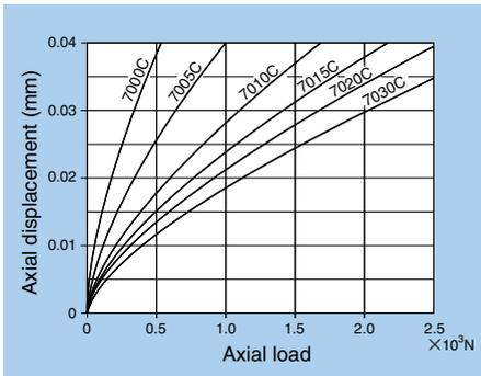
Fig. 9.5.3 Axial Load and Displacement for 70C Series
