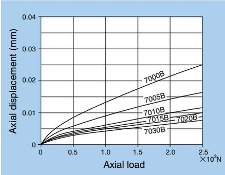
Fig. 9.5.5 Axial Load and Displacement for 70B Series
