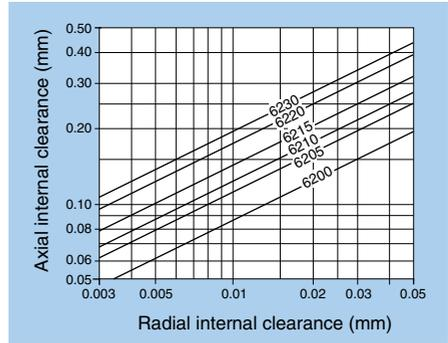
Fig. 9.4.4 Axial and Radial Internal Clearance for 62 Series
