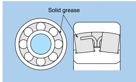
Fig. 12.2 Full pack specifications for self-aligning roller bearings
