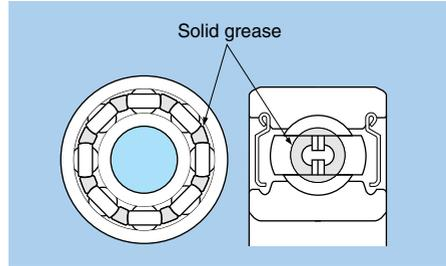
Fig. 12.1 Deep groove ball bearing spot pack specifications
