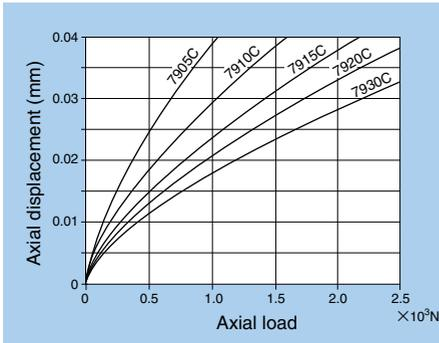
Fig. 9.5.1 Axial Load and Displacement for 79C Series
