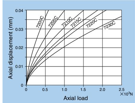
Fig. 9.5.6 Axial Load and Displacement for 72C Series
