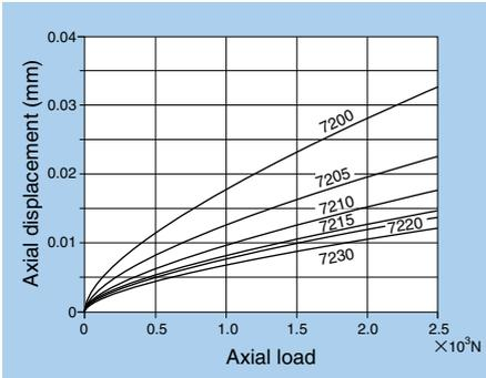
Fig. 9.5.7 Axial Load and Displacement for 72 Series
