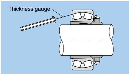
**Fig. 16.6 Measuring Internal Clearance of Self-Aligning Roller Bearings**
