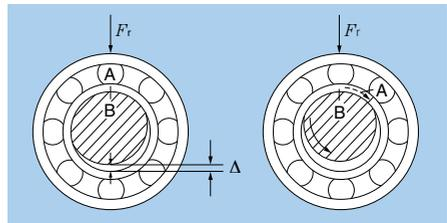
**Fig. 8.1 Bearing Creep**
