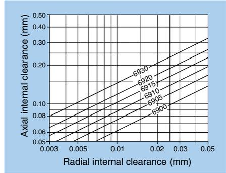
Fig. 9.4.2 Axial and Radial Internal Clearance for 69 Series
