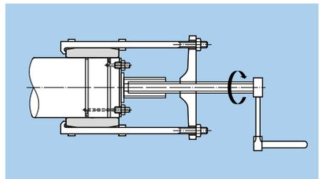
**Fig. 16.12** Removal by Hydraulic Means
