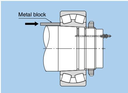
**Fig. 16.14** Removal of Bearing by Hydraulic Means
