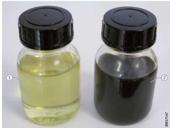
Figure 1 Change in colour of an engine oil
